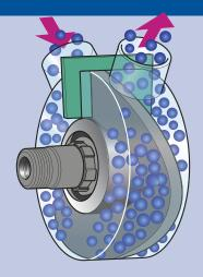
A single sinusoidal rotor creates four evenly sized chambers as it rotates. Fluid is "pulled" through the inlet into each chamber in turn. As the chamber rotates, it contracts, closes then discharges fluid through the outlet port. At the same time, the opposite chamber opens to draw in more fluid, resulting in a smooth flow with virtually no pulsation.
