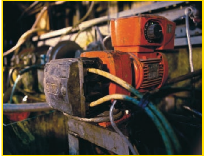
Chemically resistant 500 Series is the perfect solution for pumping corrosive cyanide in gold recovery operation
