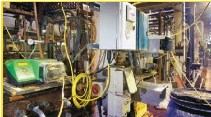
520 pump accurately meters corrosive chemicals in punishing cellulose film manufacturing process
