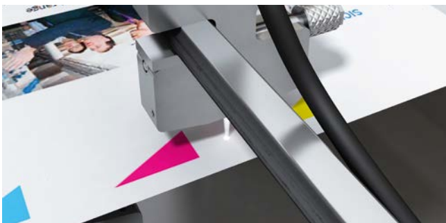
Detecting registration marks on printing machines.
