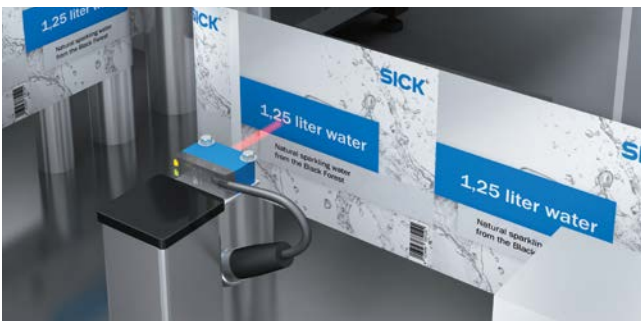
PSDI control on a packaging machine based on a color element.
