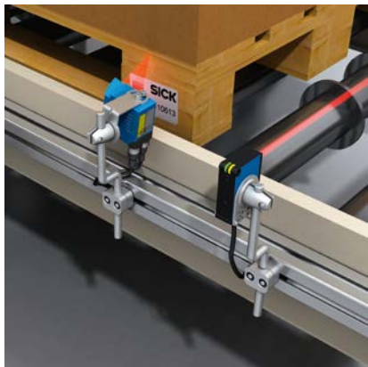
Identification of bar codes on pallet feet
