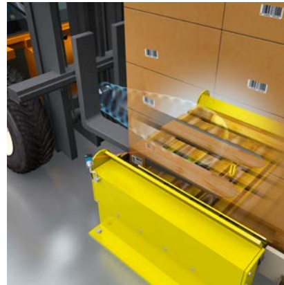
Complete tracking of the material flow using an RFID sensor on manned forklift trucks
