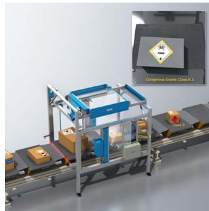
Image-based object identification with detection of hazardous material symbols
