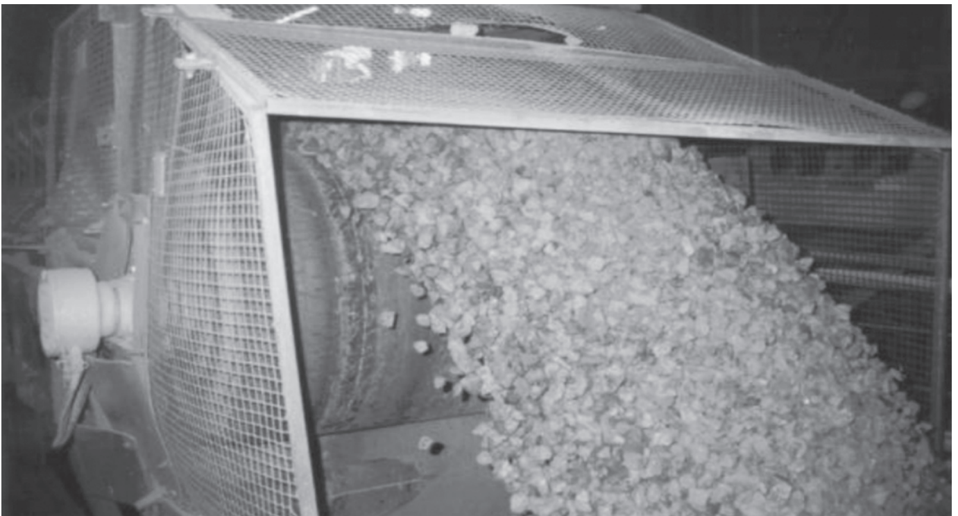
Specification: Twin drive with 2 x 800M, 37.0 kW for this travelling reversible conveyor.
