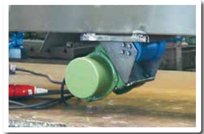
ROSTA components for pendulum mounts are mentioned in the general catalogue "Rubber suspension units".
