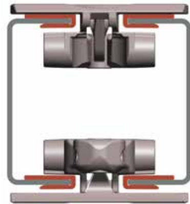
Chain width 82,5 mm (K 325) / Pitch 85 mm
