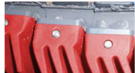
Melted flight material
