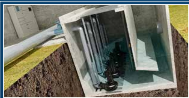
S pumps are often found in large-scale pumping stations.
