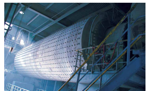
Ball mill for the cement production
