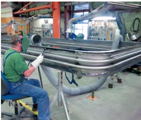
RE-type metal expansion joint with round corners being welded.
