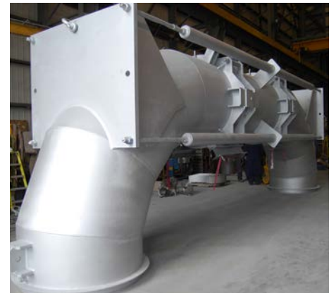
DN 1422mm refractory lined, pressure balanced expansion joint with two-ply testable bellows and test gages.
