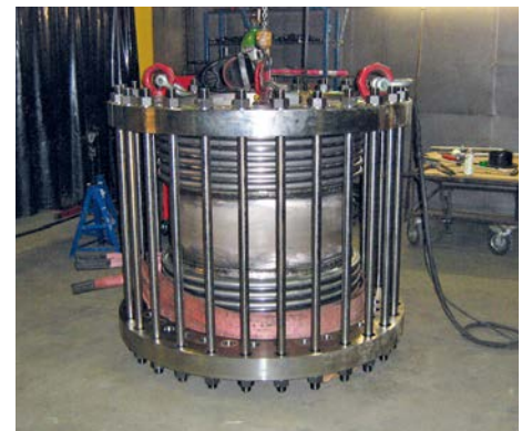
Testing a metal expansion joint with helium.
