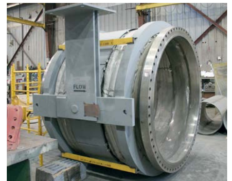
DN2000mm hinged expansion joint for a turbo expander piping system.
