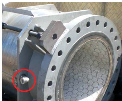
This is a typical monitoring port as it protrudes through the cover and plate.
