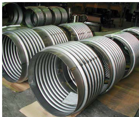
Bellows are subject to high bending stress well into the plastic range to achieve the movements required in FCC service.
