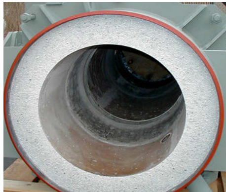
Expansion joint after being thermally dried.
