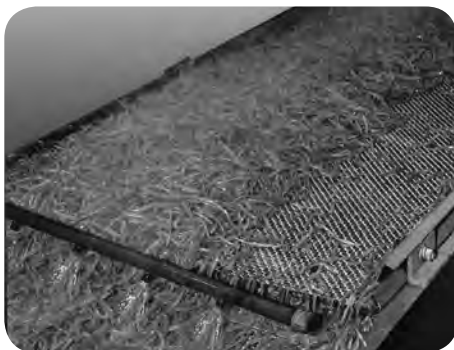
Vibrating screen being used in vegetable processing.
