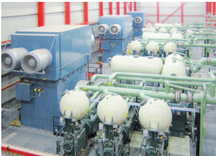
1 Azipod® propulsion unit | 2 Mine hoist motors | 3 Refiner motor | 4 Rolling mill motor (twin drive) | 5 Hydrogen gas compressor motors | 6 Medium section motors
